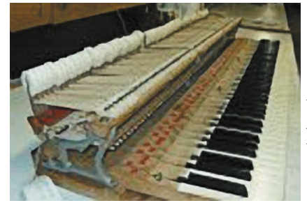
A rebuilt grand piano action with new hammers is ready for regulating and voicing.
