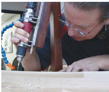
Michael Spreeman drilling holes for bridge pins
