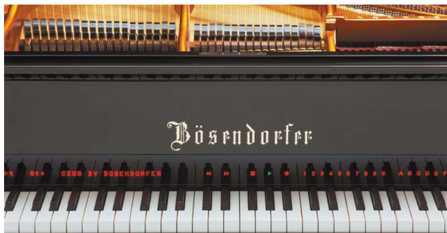
The black keys aligned with the fallboard display are among the controls used to operate the Bösendorfer CEUS.
