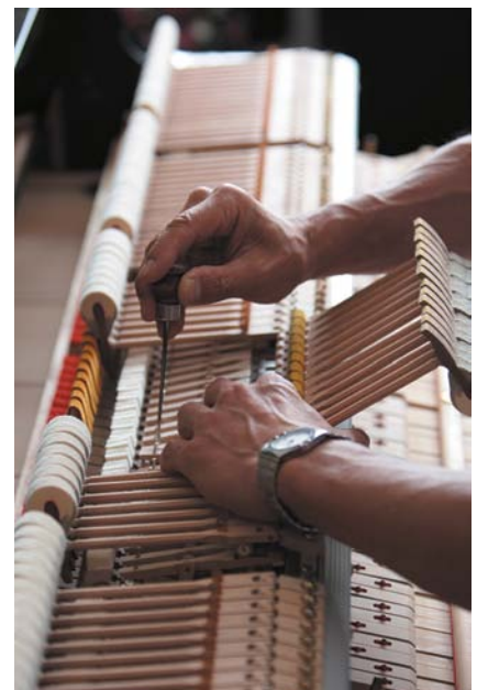
The thousands of parts in a piano action need periodic adjustment, or regulation , to compensate for wear and environmental changes.
