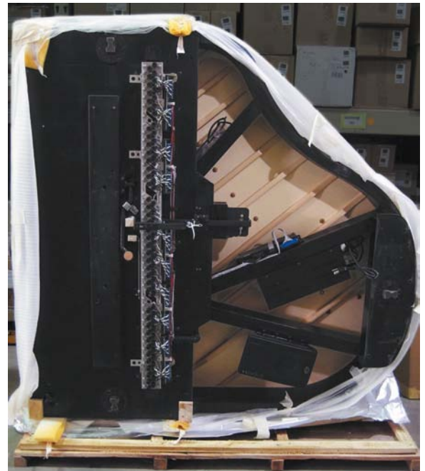
The underside of a grand piano with solenoid rail (uncovered), power supply, and speaker installed.
