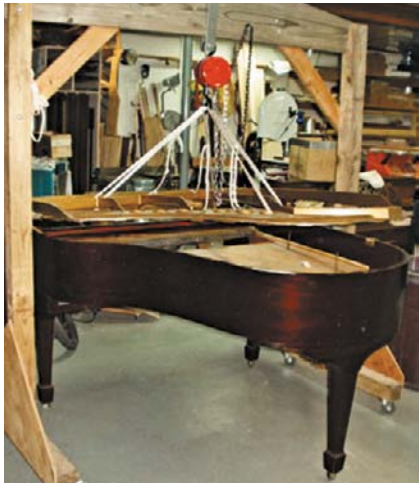
Reinstalling the cast-iron plate during the rebuilding of a grand piano
