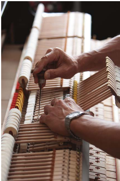
The thousands of parts in a piano action need periodic adjustment, or regulation, to compensate for wear and environmental changes.
