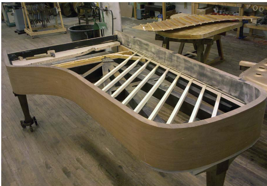
Soundboards ribs are positioned in the shelf of the inner rim, waiting to be glued to a new soundboard.
