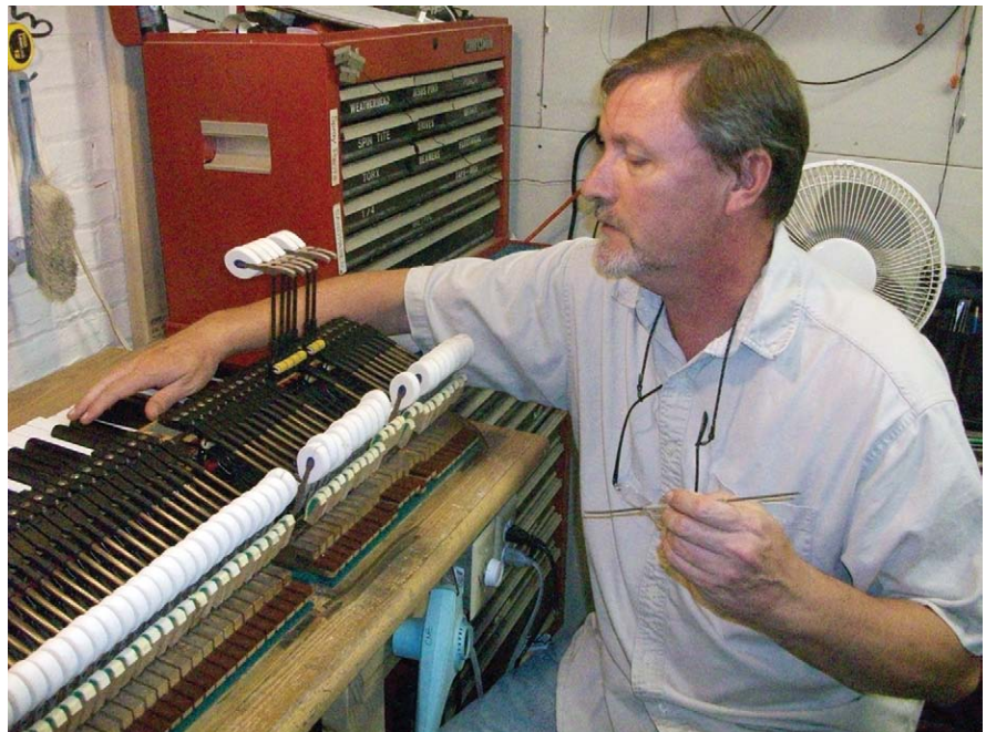
Action/Assembly department foreman Curt Brown regulating a grand piano action.
